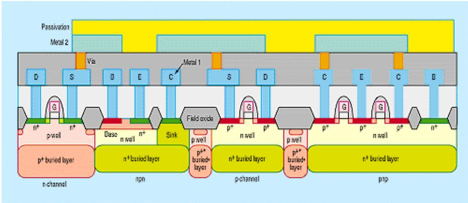
**1. The biCMOS process cross section shows nMOS, pMOS, npn, and pnp transistors. The pnp transistors are basic lateral structures formed from pMOS source/drain diffusions. The parasitic gate, which forms the base on the lateral pnp transistors, is tied back to their source.**
