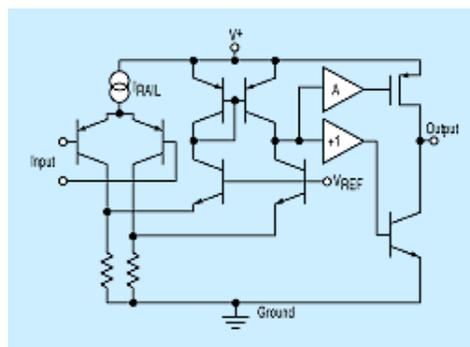
**4. To achieve well matched transistors at the input, the op amp uses PNPs instead of pMOS transistors. While the output is a combination of pMOS and npn to obtain higher output current.**
