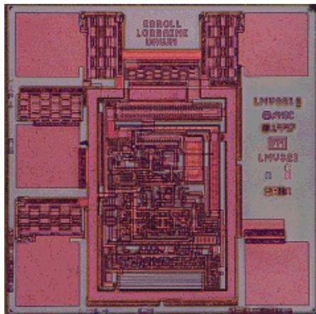
**2. The 0.8- $\mu\text{m}$  biCMOS process has shrunk the die of the LMV321 to 17 by 17 mils. And the bond pad size has been reduced to 2.8 mils<sup>2</sup>.**
