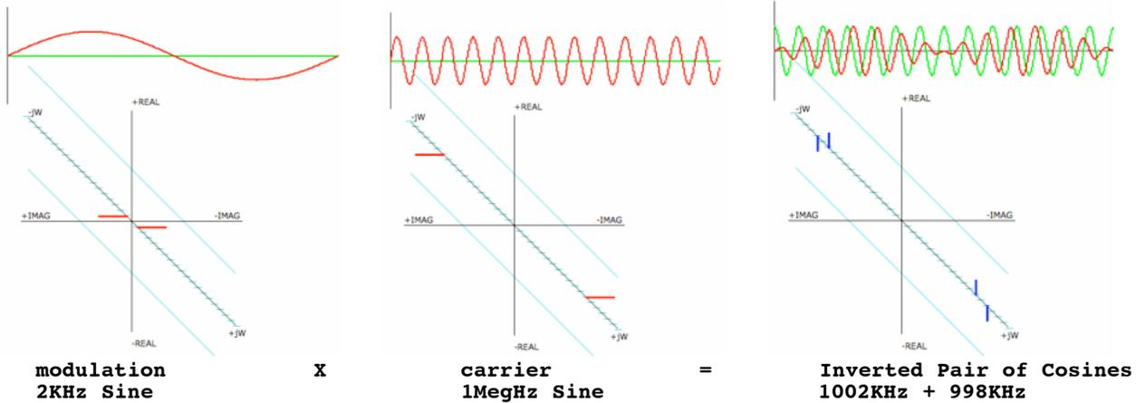
It is easy to come up with a carrier signal which is a sinewave. Suppose a filter exists that can translate any cosine audio signal into a sinewave for all frequencies.
