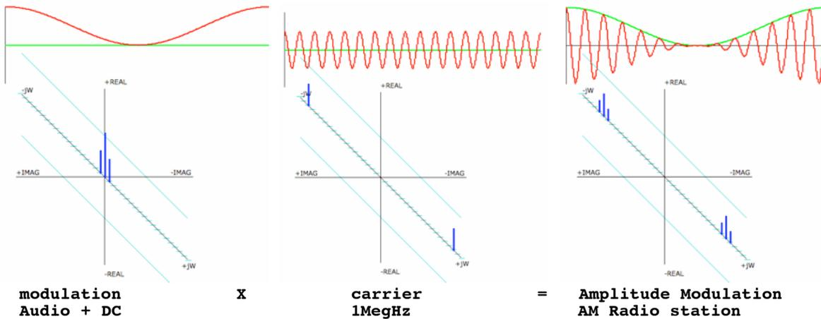
Modulation is multiplying a carrier signal by a modulation signal. Exponentials multiply by summing the power terms. The graph above shows the result of multiplying a cosine wave carrier by a cosine modulation carrier which has DC a value.
