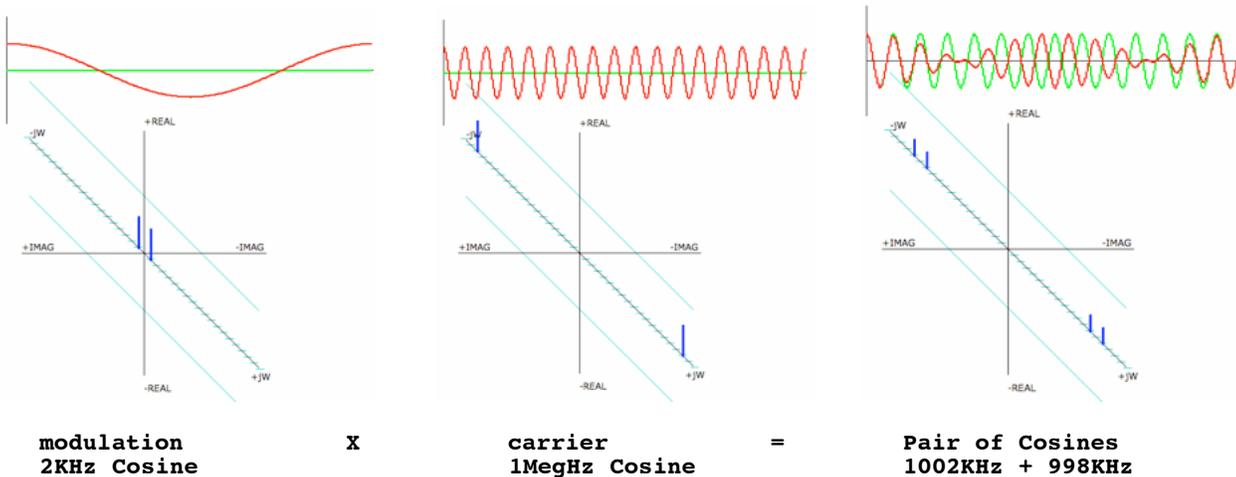
The result of multiplying a cosine wave carrier by a modulation carrier which has no DC a value is shown above. Now 100% of the broadcast energy is due to the modulation signal. The only problem is that a 2KHz bandwidth audio signal is requiring +/- 2KHz bandwidth of the broadcast band.
