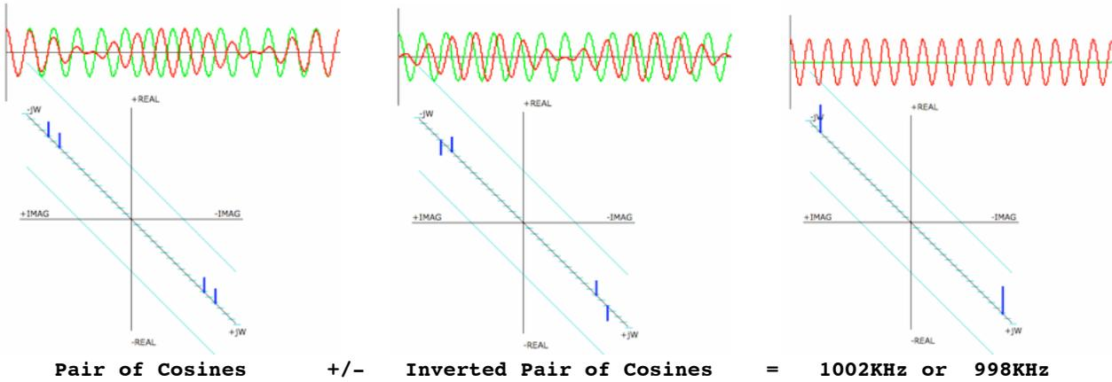
Adding or subtracting the two spectrums is going to cause one of the sidebands to cancel out. Now a 2KHz bandwidth audio signal is being broadcast over a 2KHz bandwidth at 100% efficiency.
