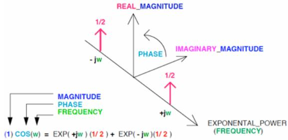
Now and again the need arises to filter a signal in a way that does not change signal magnitude, but rather changes signal phase. The price of bandwidth has always been expensive. Single sideband modulation is an old method of broadcasting a signal efficiently. The Euler identity equation provides a good way of mapping AC signal into a 3 dimensional graph to make it much easier to see how this is done.
