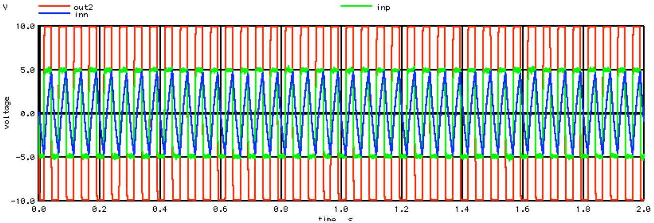
The Noise source **BPWL** can be seen on the **inp** input. But its PM effects are hard to see. A spectrum can show the details.
