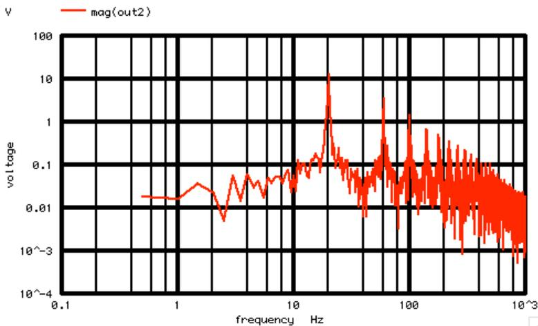
The actual noise is appearing close to the peak signals at 20Hz and 60Hz and 100Hz, etc. Since white noise was applied, the slope of the adjacent noise sidebands around 20Hz drop in power to the  $1/f^2$  as they get farther away from 20Hz. The same is true for all the odd harmonics.
